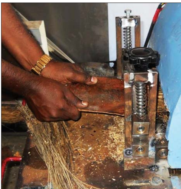
Springs fitted in columns
