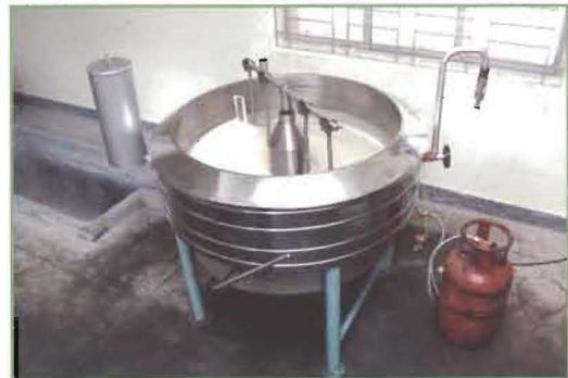
Fig. 8. Hot processing of VCO in VCO cooker
