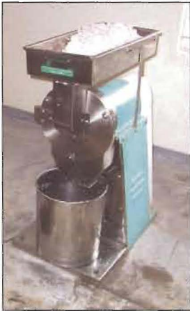
Fig. 5. Mechanical Coconut grating machine/Coconut pulverizer
