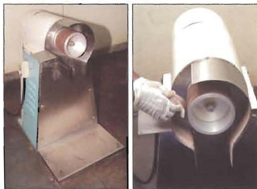
Fig. 4. Testa removal using testa remover
